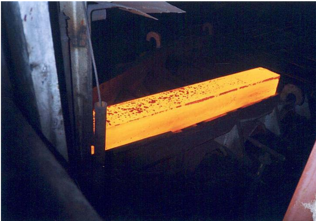
Photo below: This billet has been descaled with high pressure water. The dark marks which can be seen on the glowing steel are water drops only.
