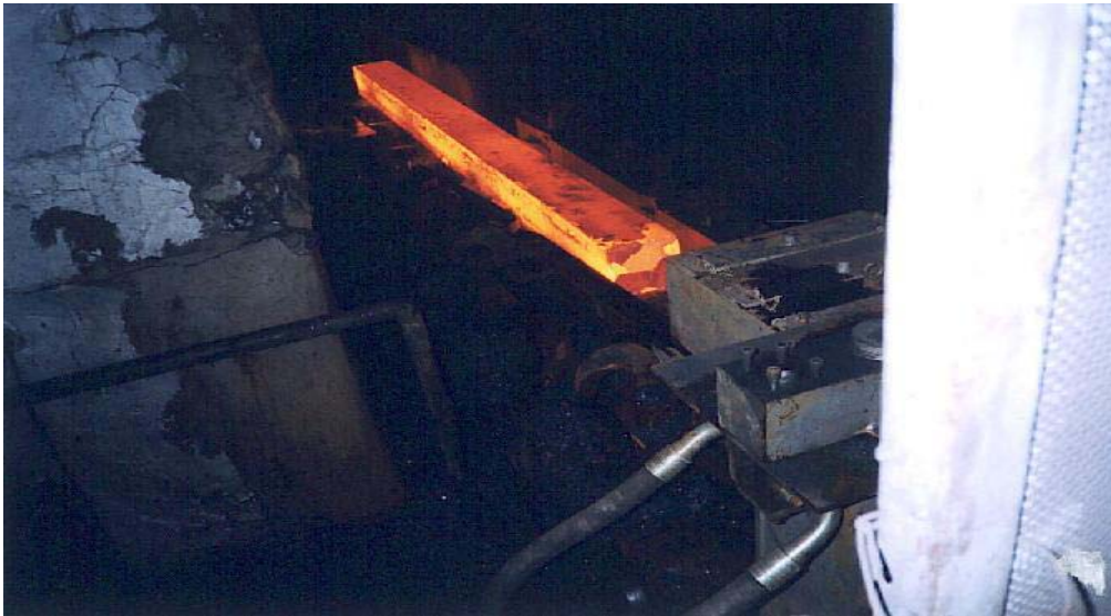
Photo above: On the billet leaving the furnace the scale is clearly visible
