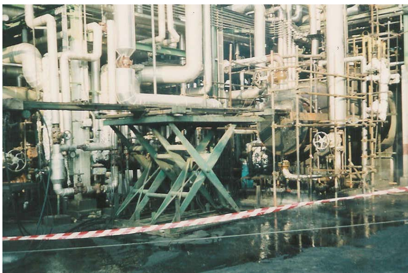
Scissor-type lifting table with lance unit for internal cleaning
