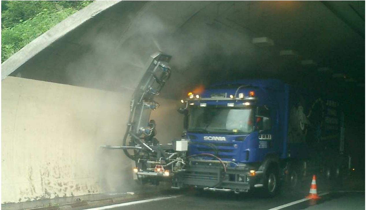
Photo above: The purpose-built vehicle TCT 400 H during operation. The nozzle arrangement at the front of the vehicle can be configured hydraulically to match the tunnel profile
