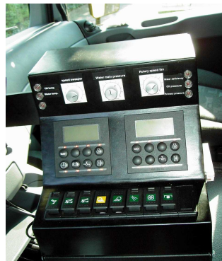
Additional control panel in driver's cab
