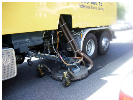
Surface cleaner with suction device in working position
