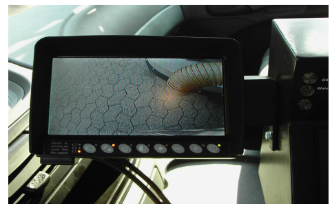
Monitor in the driver's cab for transfer of the cleaning results
